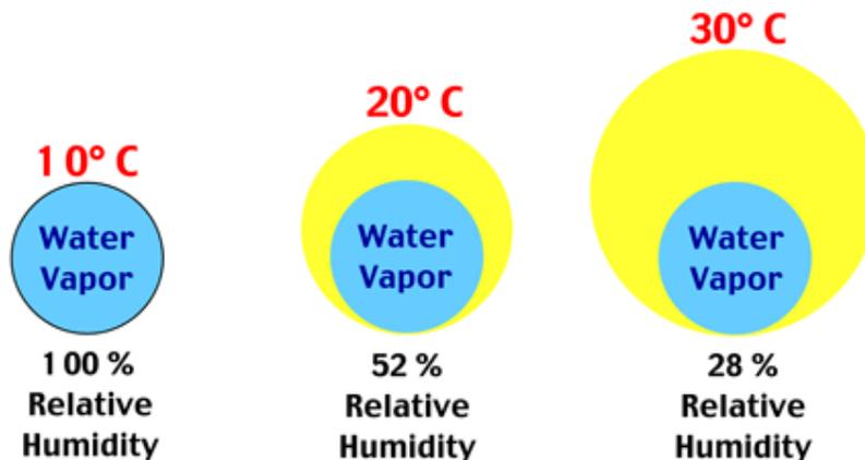
The diagram above illustrates how relative humidity changes in a parcel of air with increases in air temperature. At 10°C a parcel of dry air weighing one kilogram can hold a maximum of 7.76 grams of water vapor. In this state, the parcel of air would be at saturation (dew point) and its **relative humidity** would be **100%**.
